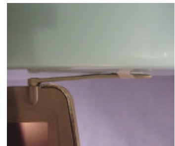
Body SAR Test Setup 0.25cm Separation Distance
