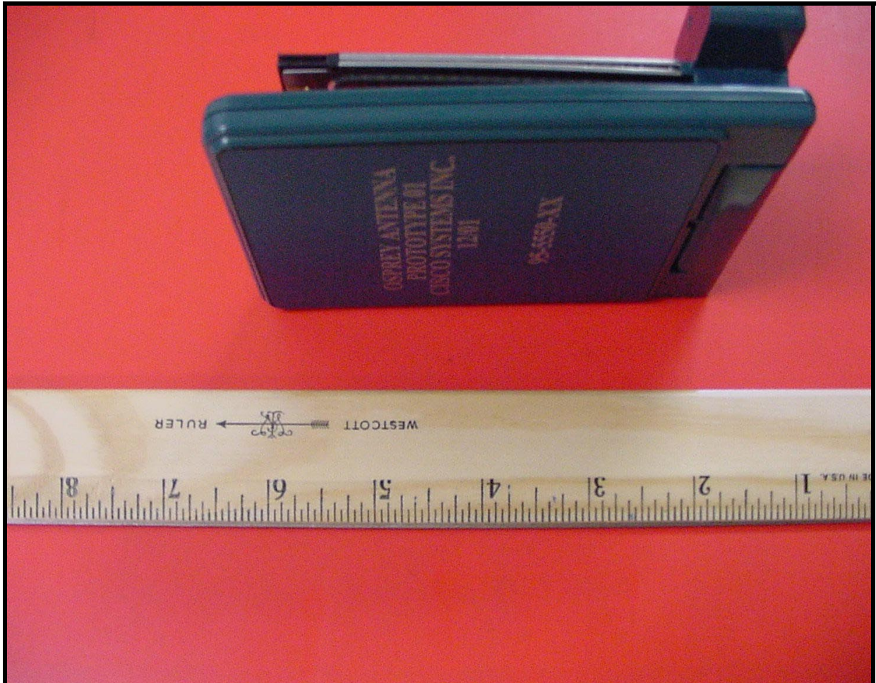
PHOTOGRAPH 8: 5GHZ TX MODULE WITH INTEGRAL ANTENNA
