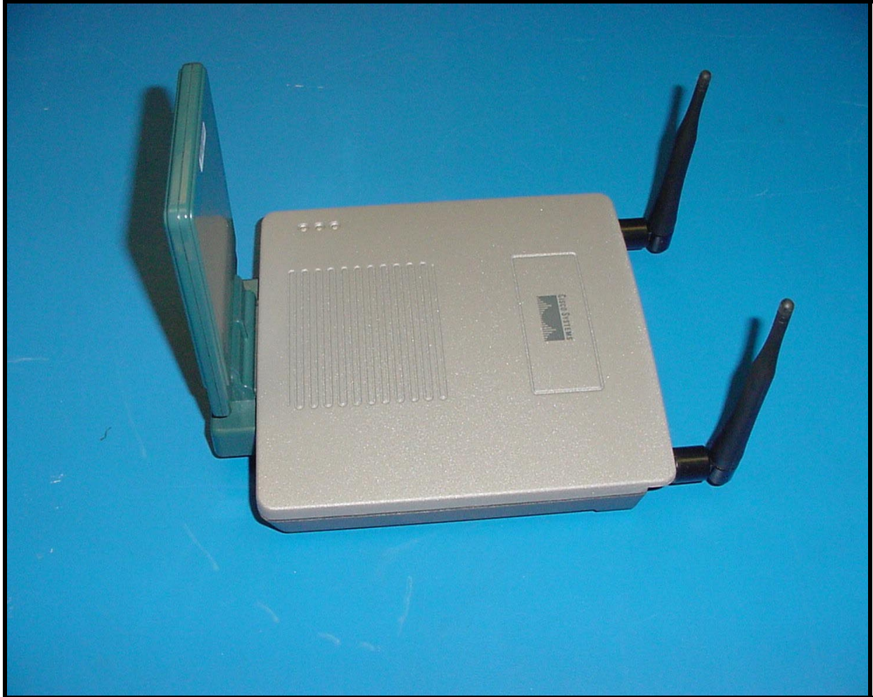
PHOTOGRAPH 5: AP1200 WITH 2.4GHZ AND 5 GHZ TX MODULES
