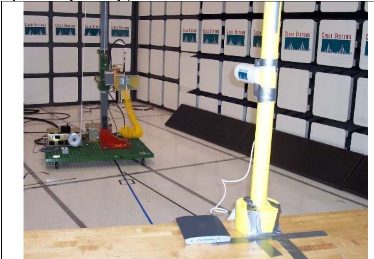
Title: 18-40GHz Radiated, 2.4GHz 10dBi Yagi Antenna
