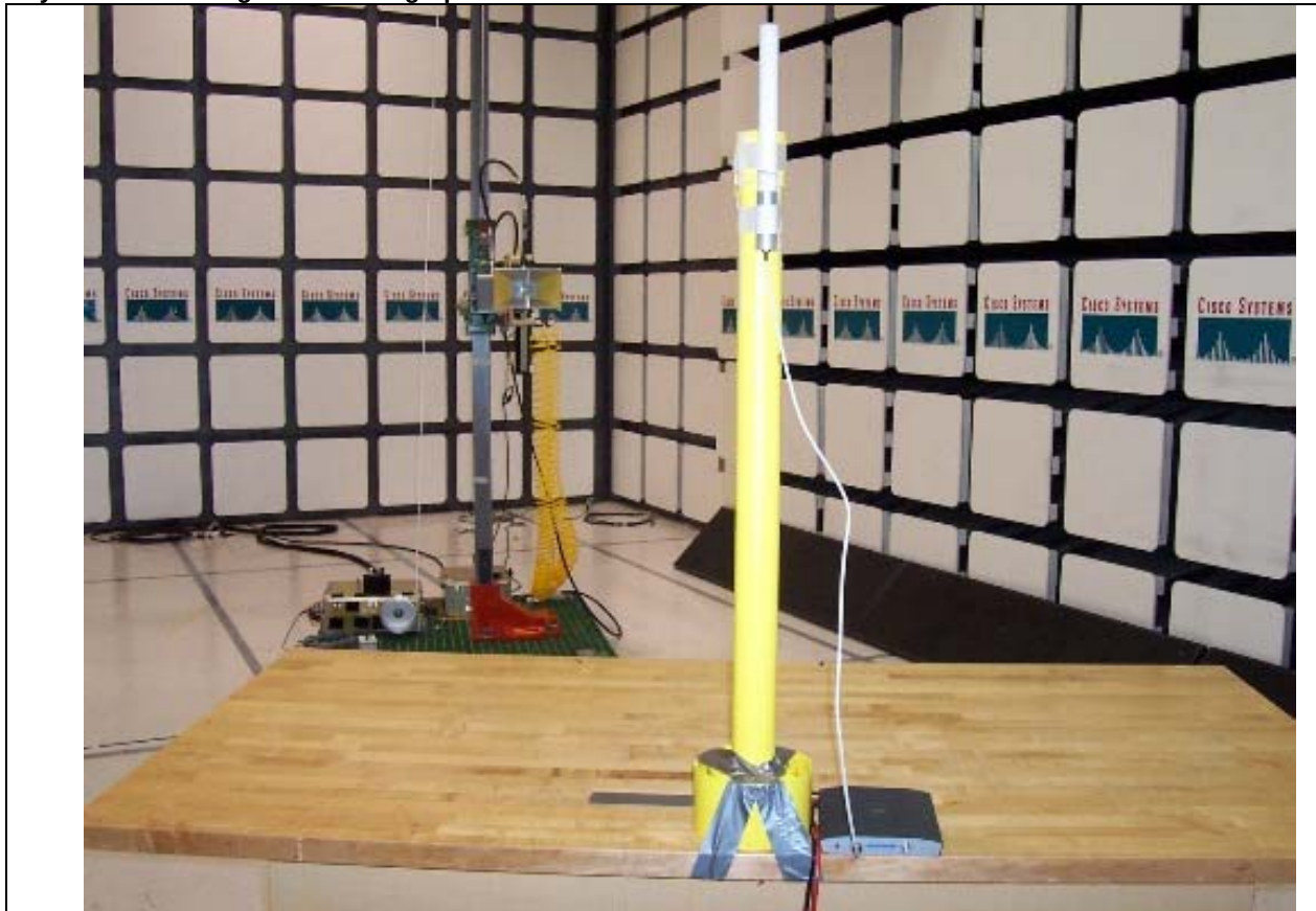
Title: 1-18GHz Radiated, 5GHz 6dBi Omnidirectional Antenna
