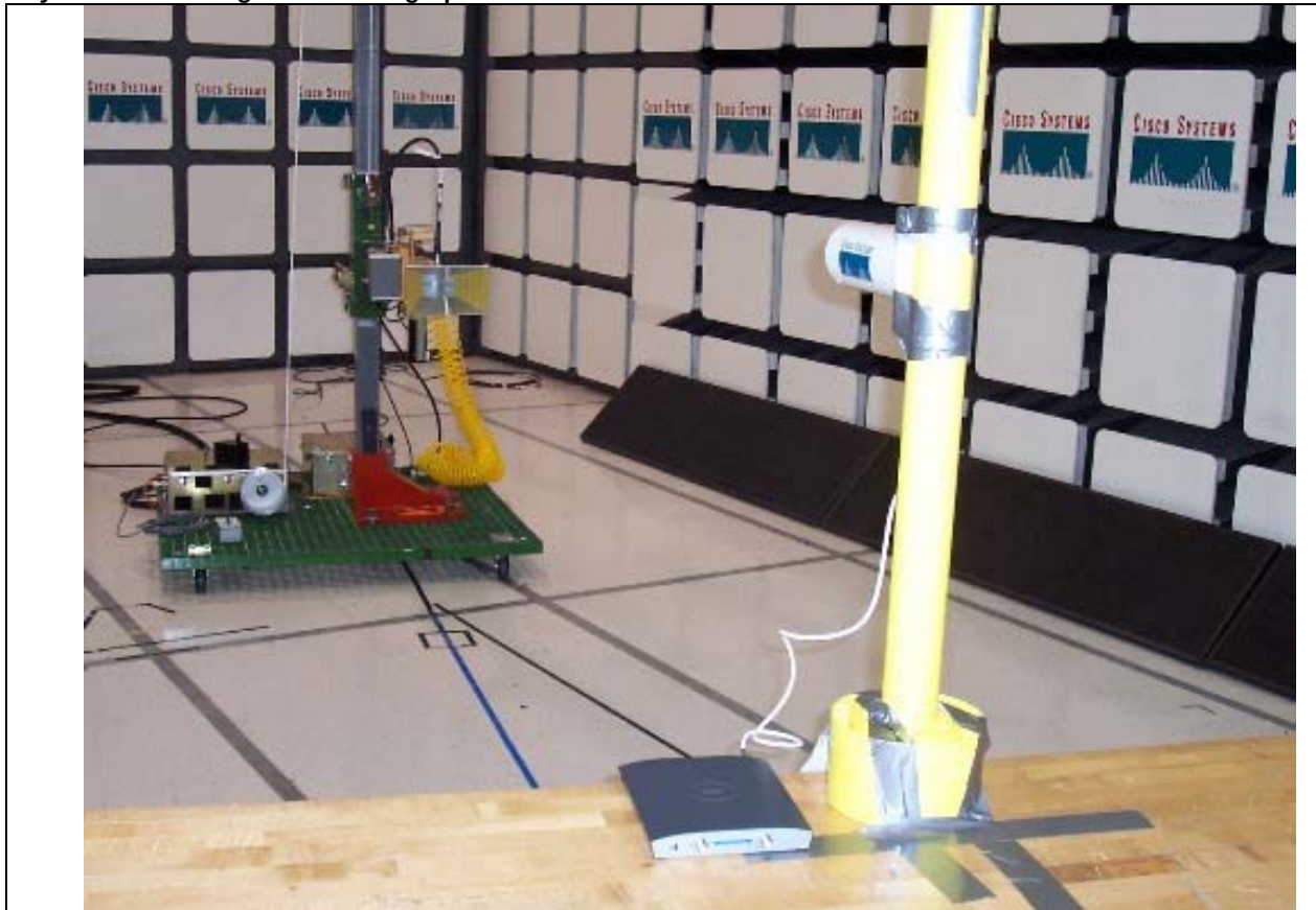
Title: 1-18GHz Radiated Setup, 2.4GHz, 10dBi Yagi Antenna
