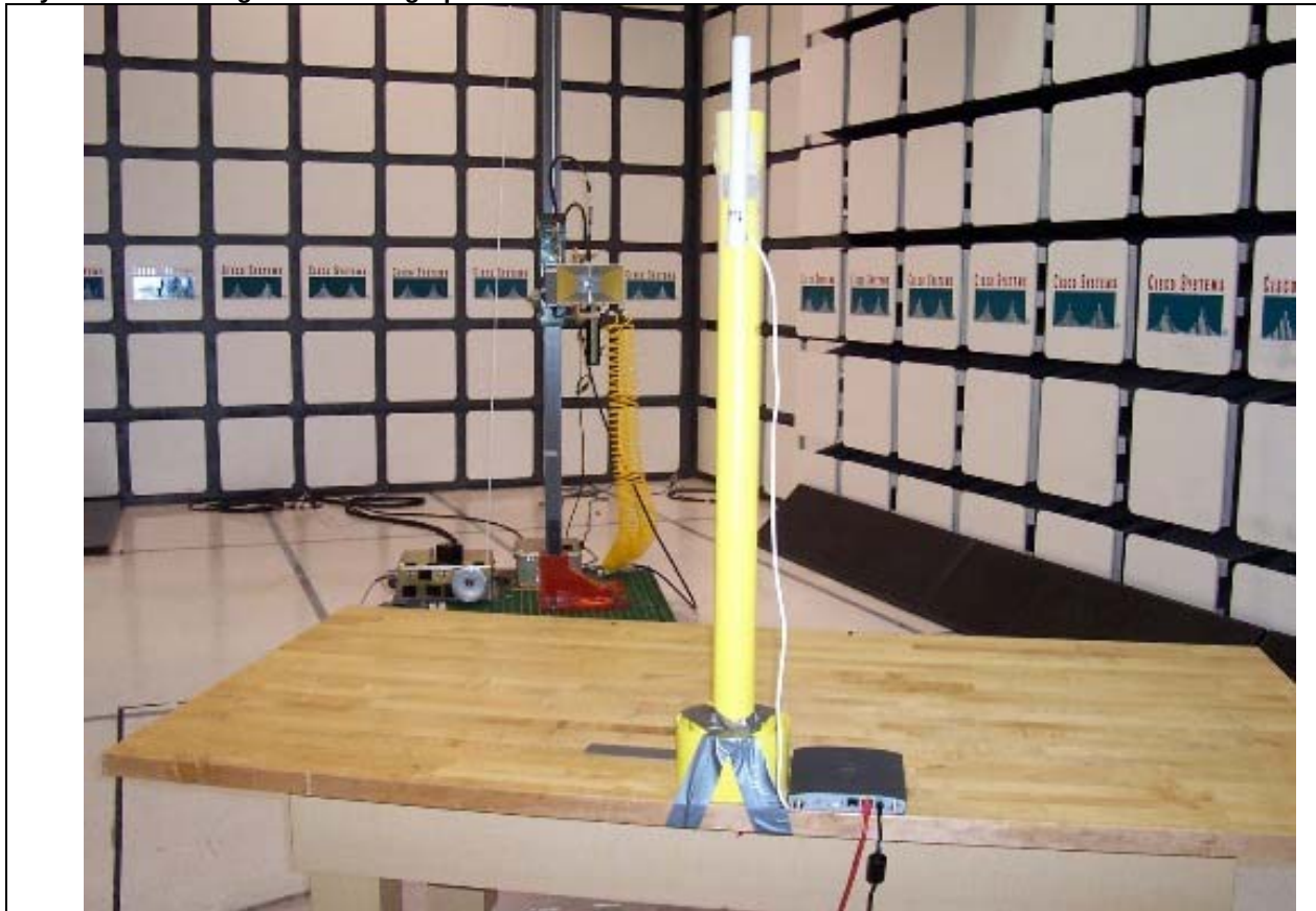
Title: 1-18GHz Radiated Setup, 2.4GHz 5.2dBi Omnidirectional Antenna
