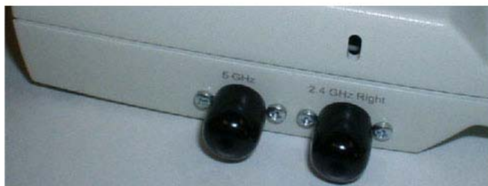
B. 5 GHz/802.11a and 2.4 GHz/802.11b Right External Antennas
