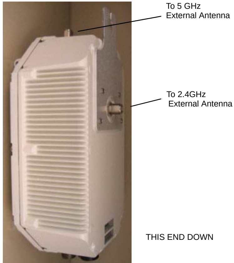
Figure 3-8 Optional Outdoor Access Point and Antenna Orientation
