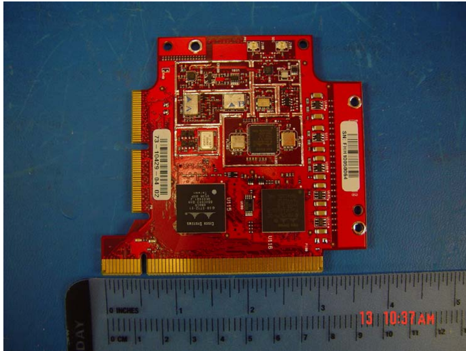
AIR-RM1251G Top with Shields Removed
