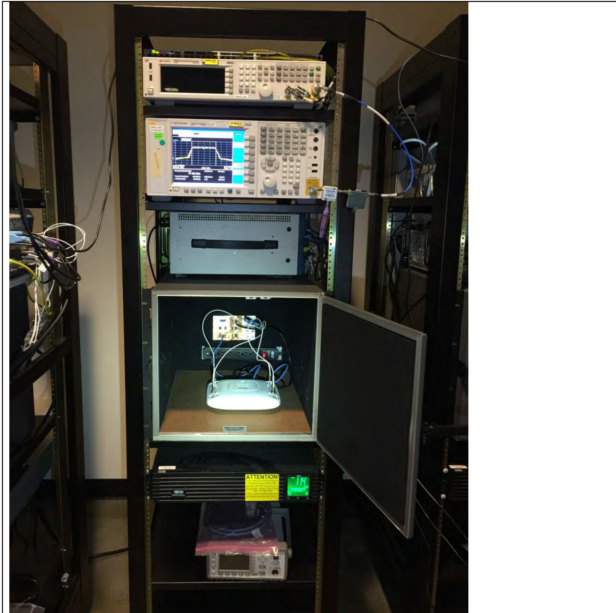
Title: AIR-CAP2602E-B-K9 Physical Test Arrangement Photograph
