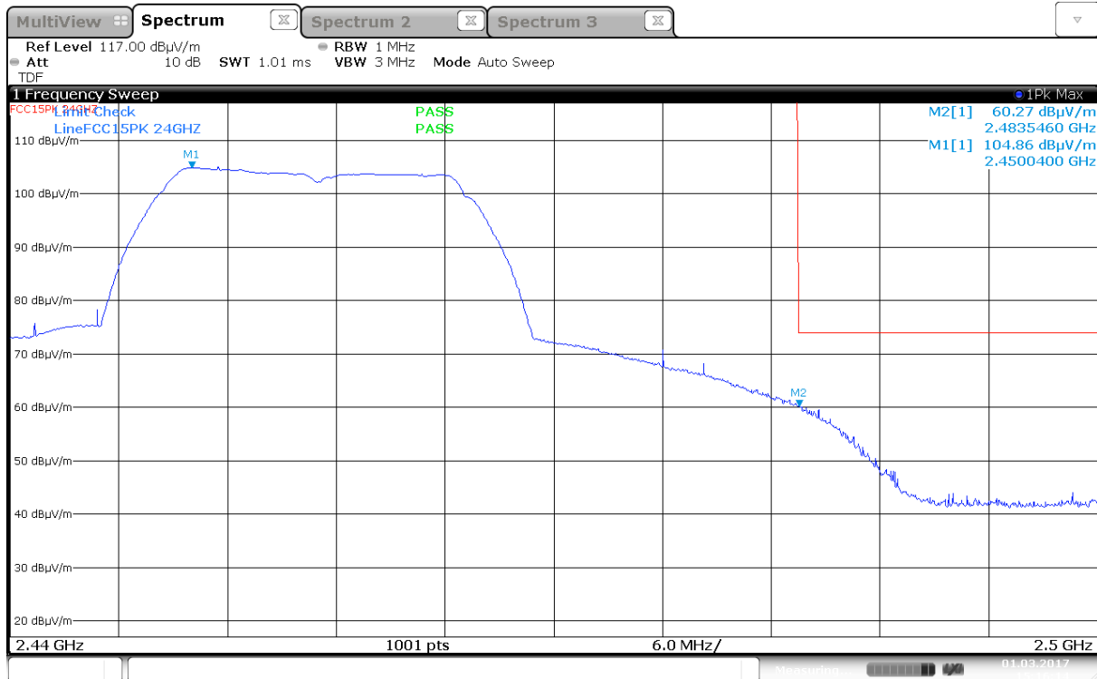
Upper Band Edge, Peak, 2457 MHz, 802.11g, 6Mbps, (Max: Ant 0, HP)
