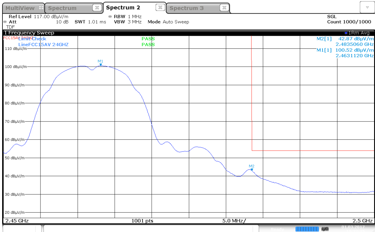
Upper Band Edge, Average, 2462 MHz, 802.11b, 1Mbps, (Max: Ant 0, HP)
