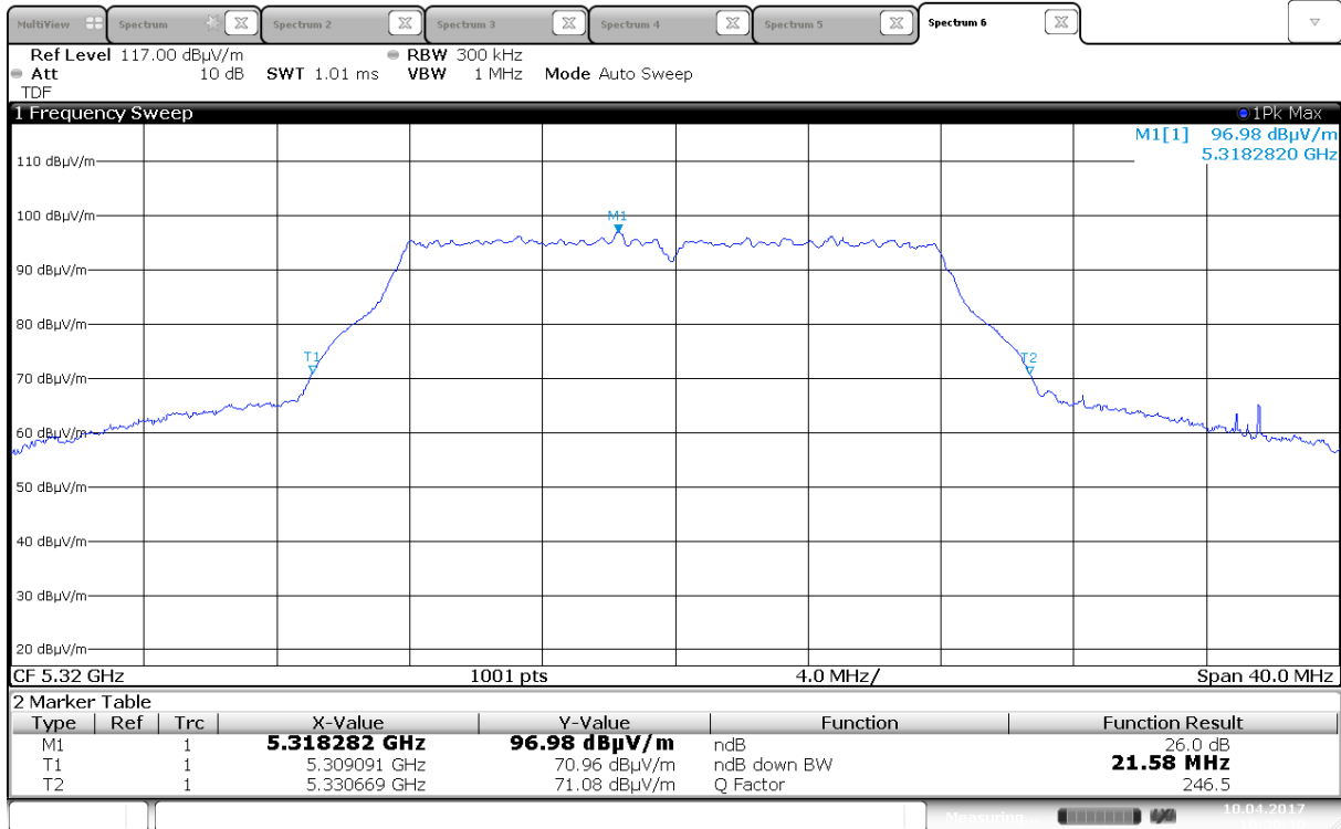
Emission Bandwidth B, 5320 MHz, 802.11a 6Mbps, Ant 0
