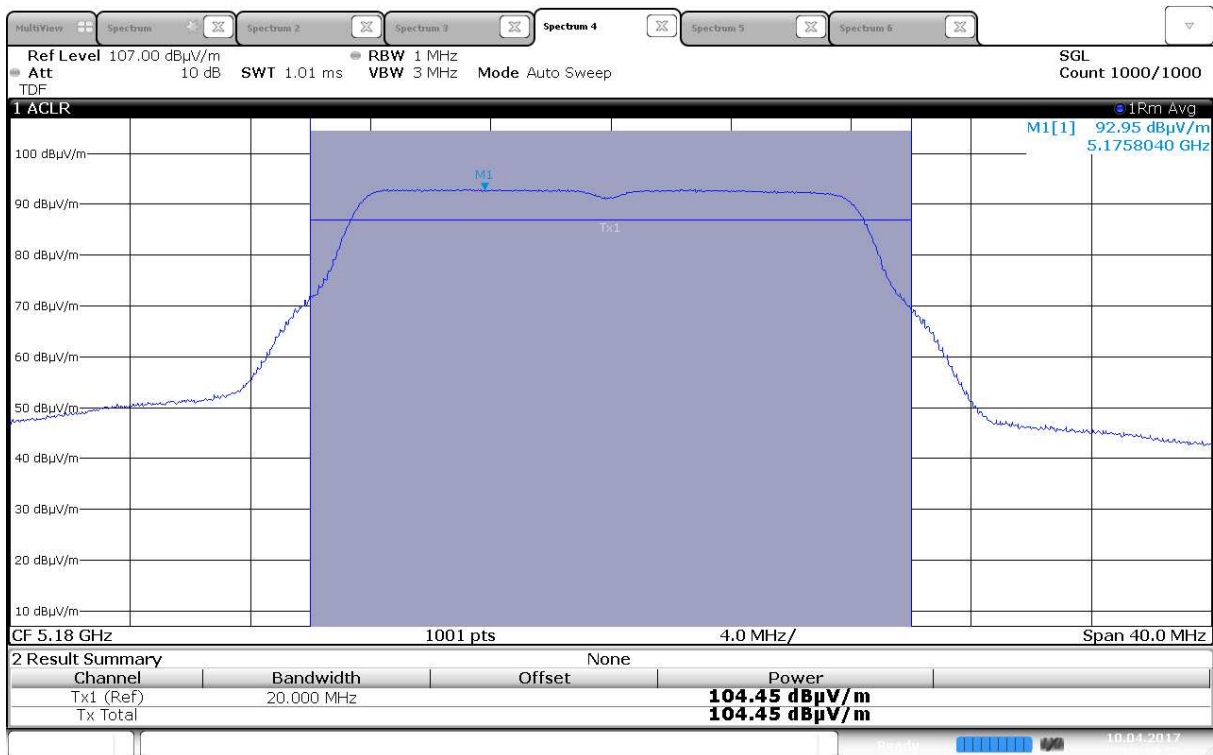
Maximum EIRP, 5180 MHz, 802.11a 6Mbps, Ant 1
