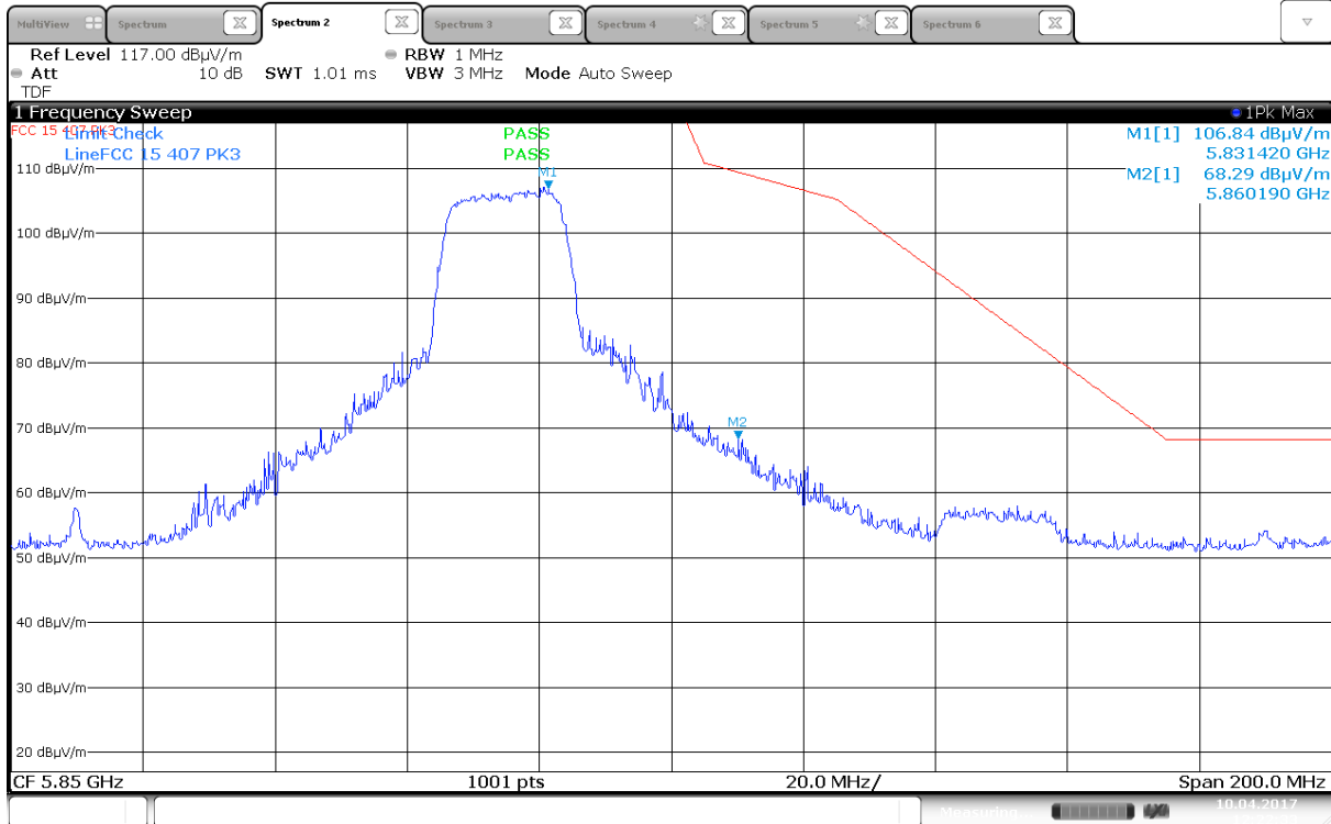
Unwanted Emissions, Band Edge, 5850MHz, ch165, 802.11n MCS0 HT20, MIMO
