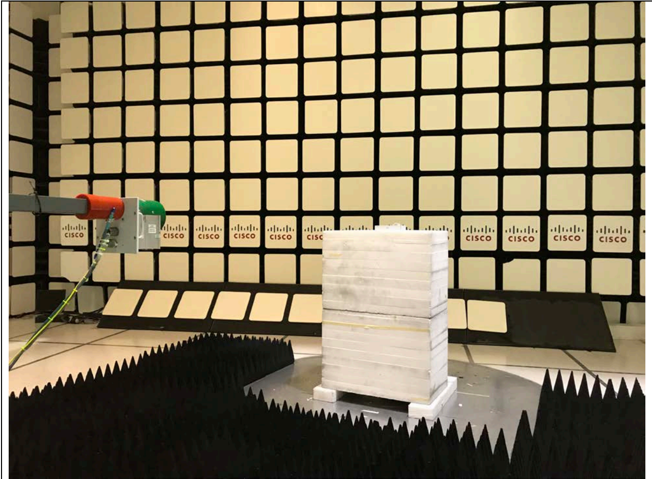
Title: Radiated Emissions 18-40GHz Configuration Photograph
