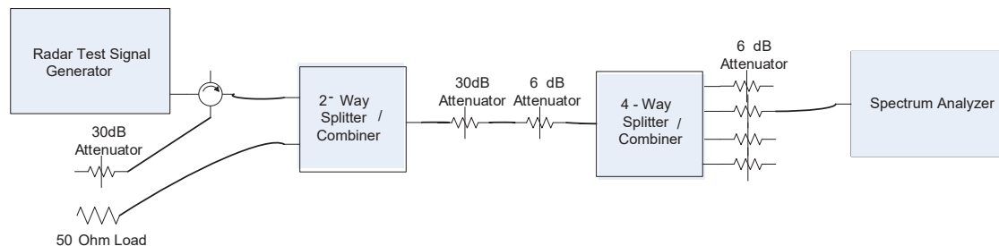
Conducted Calibration Setup
