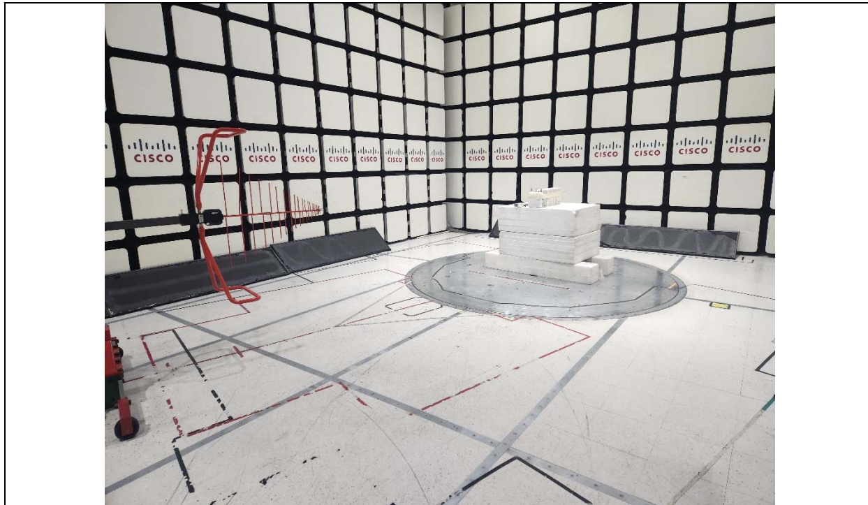
Title: 5GHz & BLE Radiated Spurious Emissions Test Configuration 30M - 1000MHz
