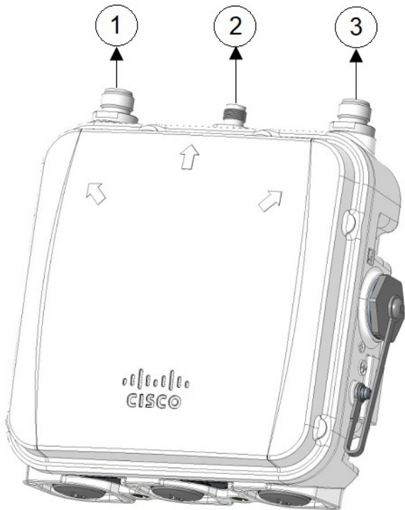
Figure 3: IW9165D Top Connectors and Ports
