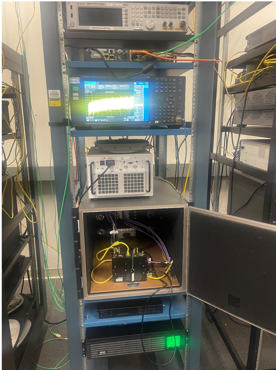
IW9165E-B & IW9165E-A Conducted test setup picture
