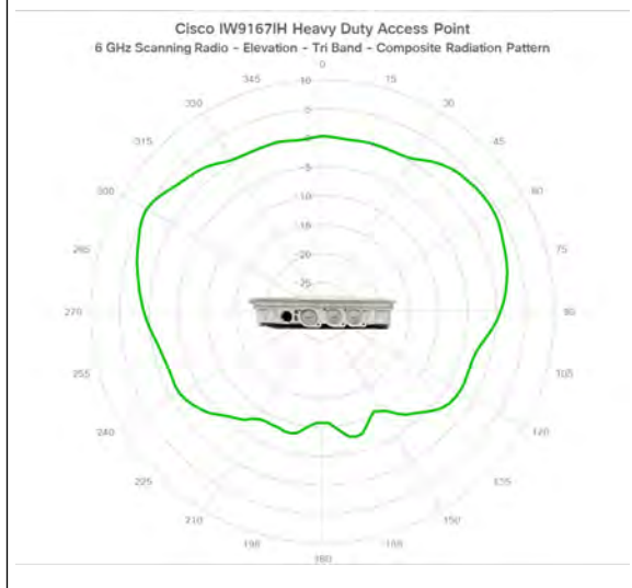
Figure 18: IW9167IH - Scanning Radio - Tri Band Composite Radiation Pattern (6-GHz Elevation)
