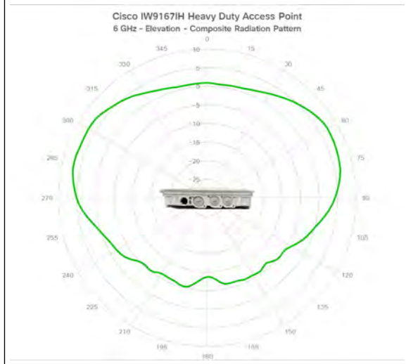
Figure 10: IW9167IH - Composite Radiation Pattern (6-GHz Elevation)
