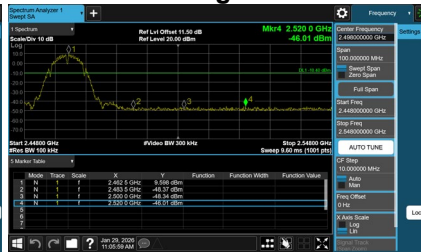
CH01 – 10th Harmonic of the fundamental frequency
