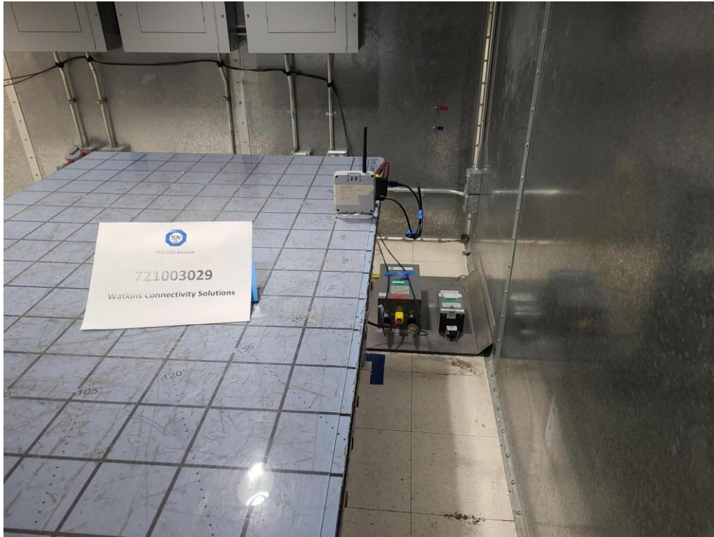
AC Mains Conducted Emissions Test Setup - HNA
