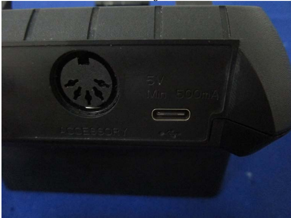
EUT – Base Charger Port View
