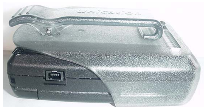
Right Side of Belt-Worn Holster with DUT (plastic with metal screw)
