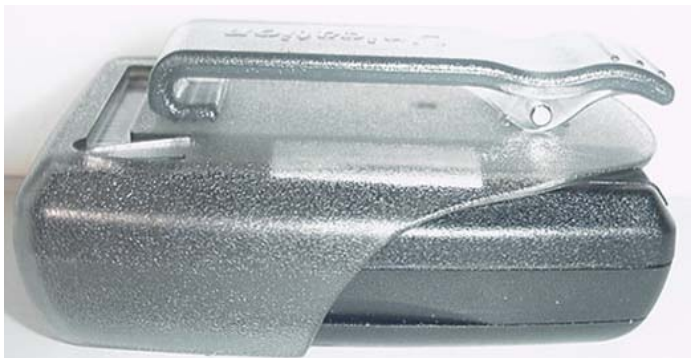
Left Side of Belt-Worn Holster with DUT (plastic with metal screw)
