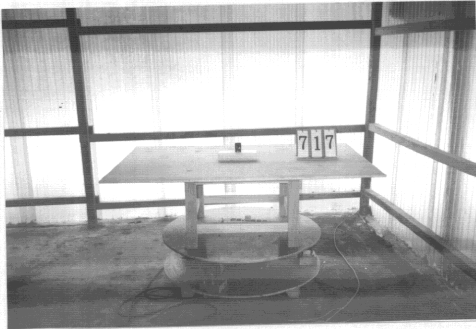
Fig 1. Test Configuration of the Radiated Emissions (Front View)
