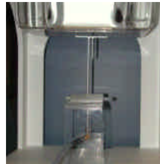
Figure A.0 Dipole Validation Test Setup
