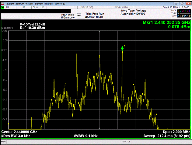
BLE/GFSK 125 kbps Mid Channel, 2440 MHz
