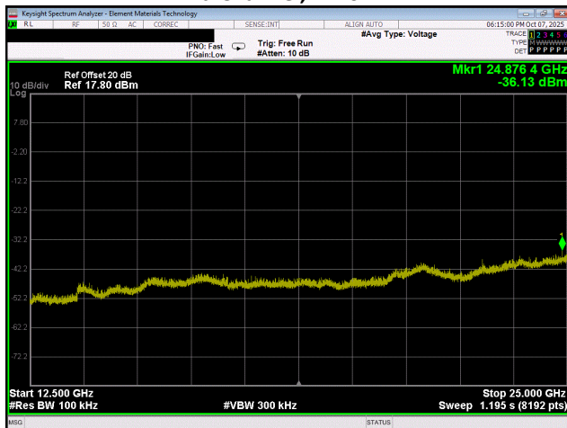
BLE/GFSK 1 Mbps Mid Channel, 2440 MHz
