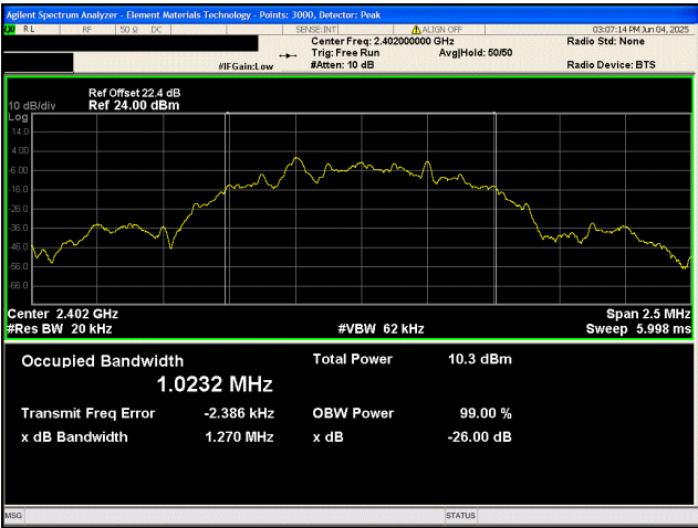
BLE/GFSK 500 kbps Low Channel, 2402 MHz
