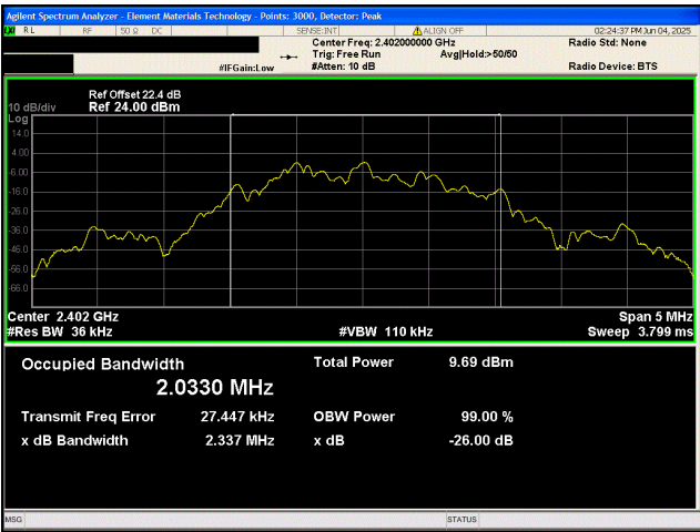
BLE/GFSK 2 Mbps Low Channel, 2402 MHz
