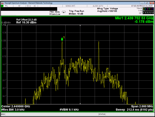
BLE/GFSK 500 kbps Mid Channel, 2440 MHz
