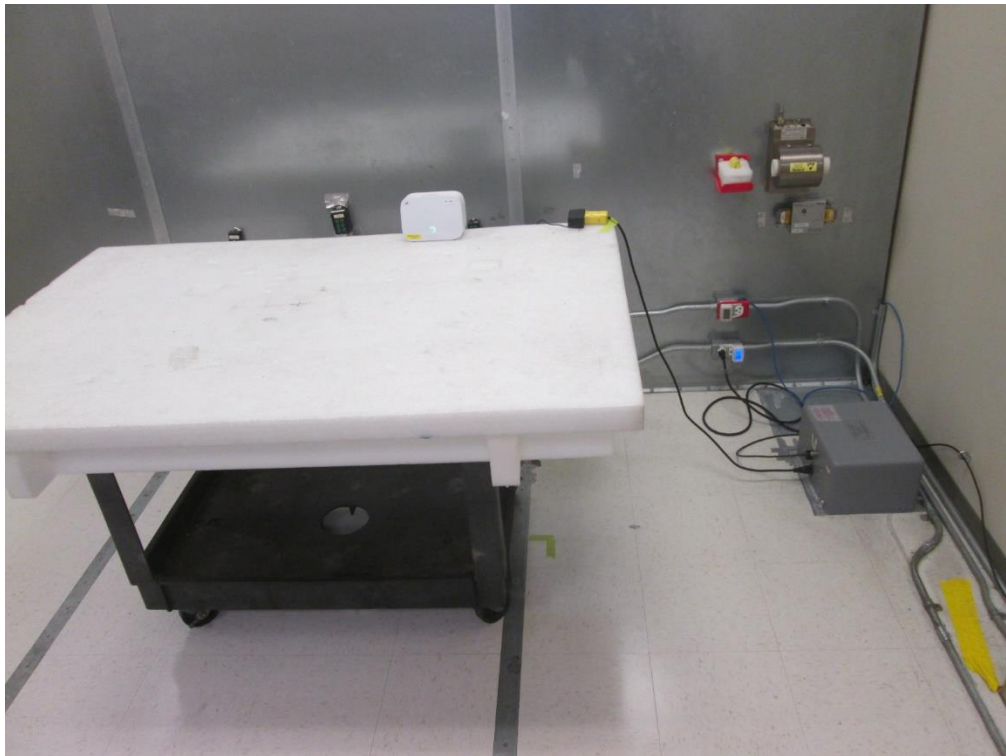
Power Line Conducted Emissions
