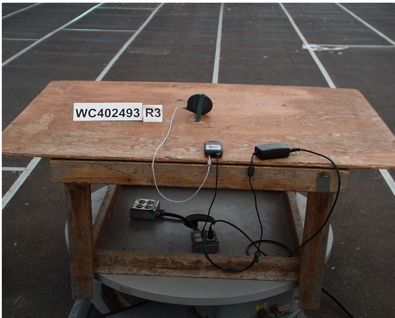
Test-setup photo(s): Radiated emission 10 kHz - 1000 MHz
