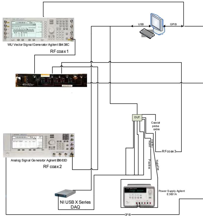
Figure 10 Test setup for Rx spurious response rejection testing
