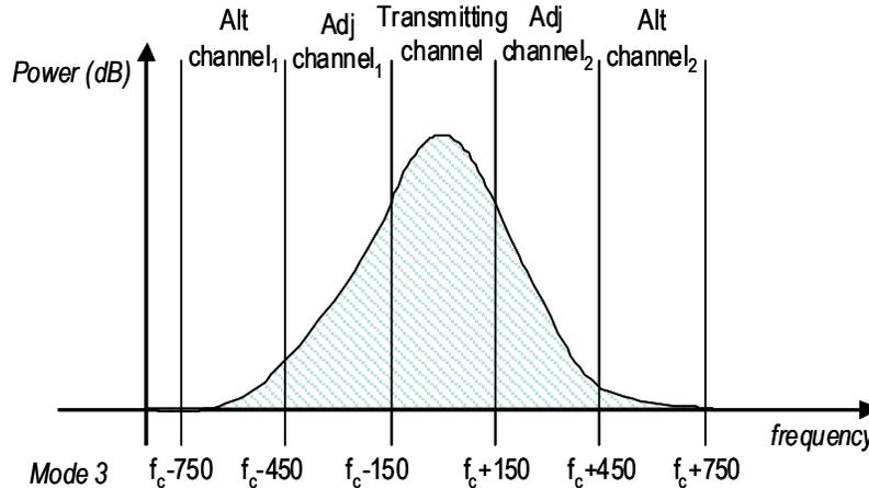
Figure 26. Mode 3 Transmit Channel Illustration
