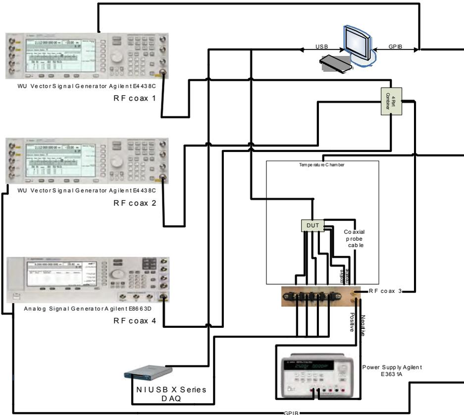
Figure 2. Test setup for receiver testing
