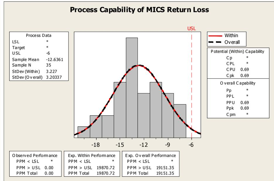
Figure 37 Capability Analysis of Return Loss
