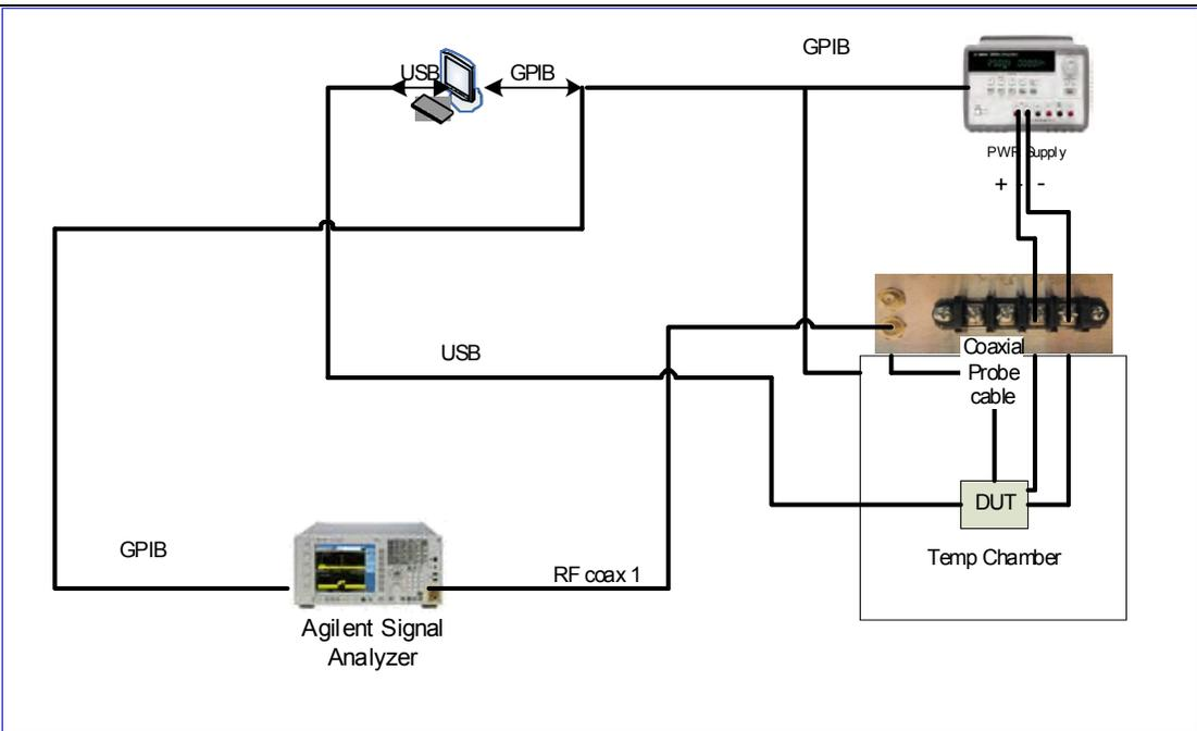
Figure 27 Test setup for Tx testing
