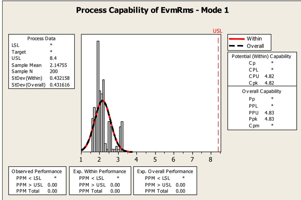
Figure 31 Capability Analysis of Error Vector Magnitude
