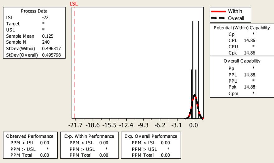
Figure 4 Capability Analysis of Mode 1 Upper Dynamic Range Level
