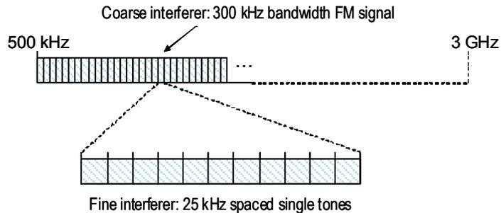
Figure 9. Diagram of interference strategy for single tone spurious harmonics test.
