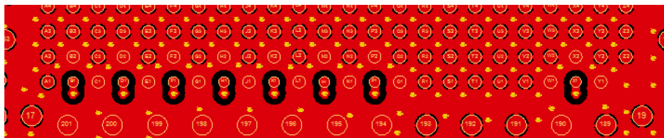
Figure 9-3: Antenna Pad Ground Cutout Recommended (Main Board, top layer/NAD side)
