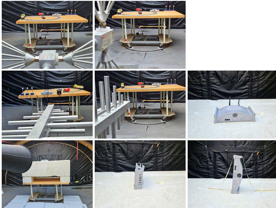
Figure 4: Radiated Emissions Test Setup Photograph(s).
