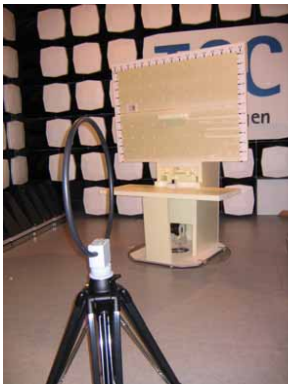
Picture 1 Radiated emission measurement 9 kHz to 30 MHz
