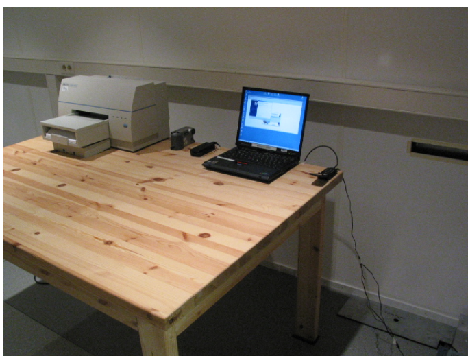
Picture 4 AC powerline conducted emission measurement WLAN TX + Computer peripherals
