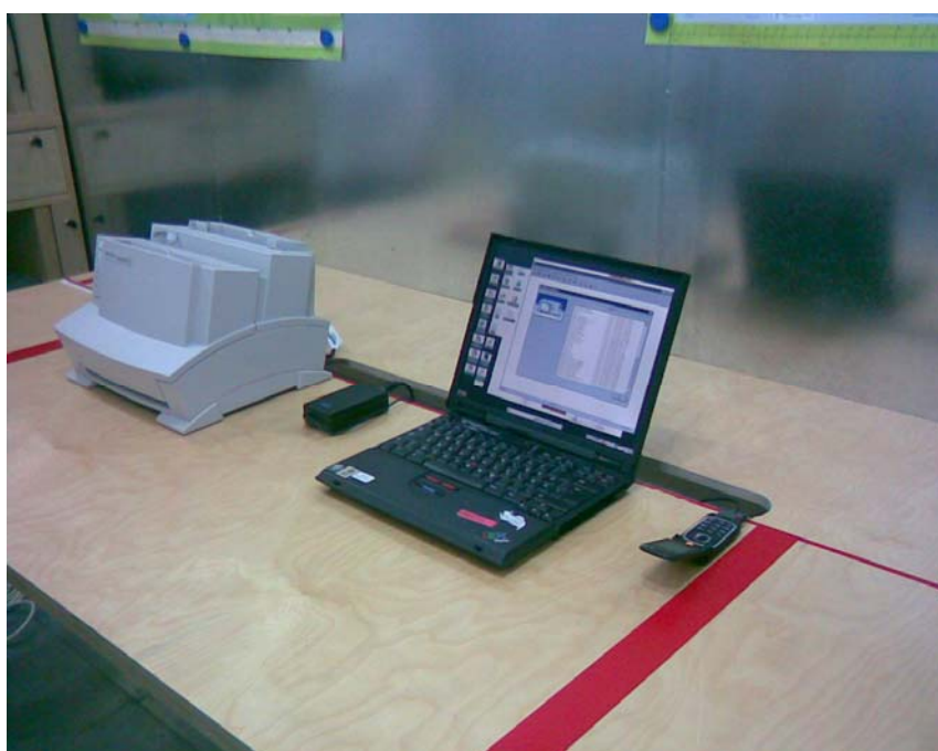
Picture 4 AC powerline conducted emission measurement GSM RX/Bluetooth TX + Computer peripherals
