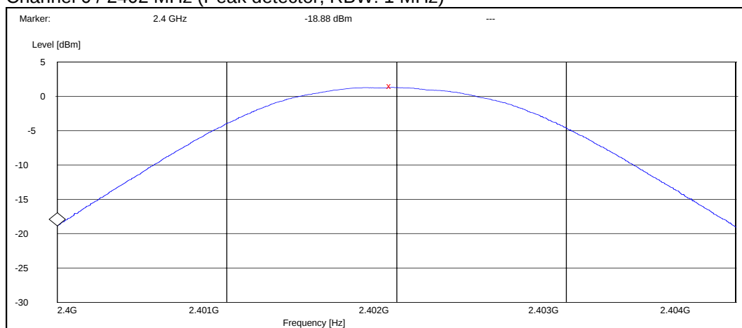
Channel 0 / 2402 MHz (Peak detector, RBW: 1 MHz)
