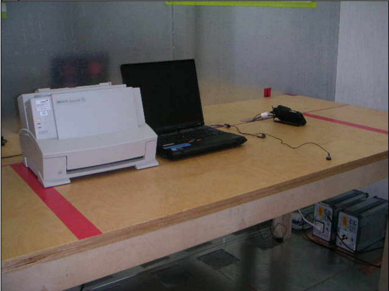
Picture 3 AC powerline conducted emission measurement Bluetooth RX + Computer peripherals
