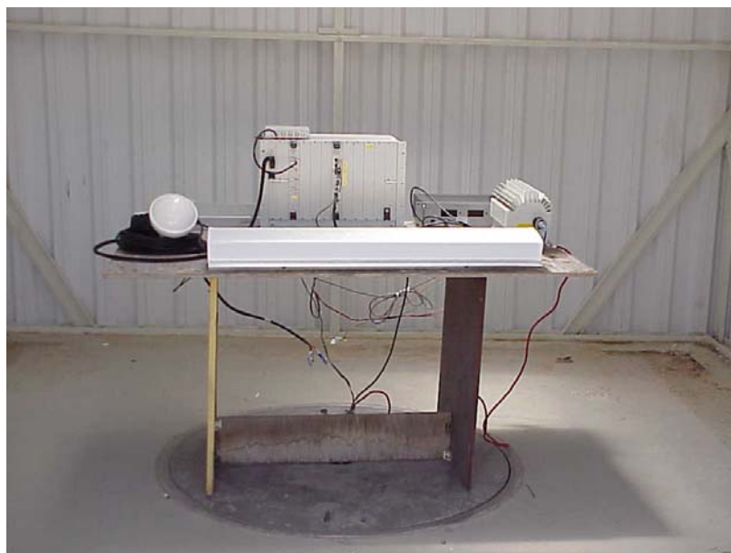
Photo 2. Indoor unit. Test setup on OATS
