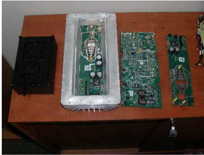
Photo 3. High power amplifier, cavity filter, base unit PCB.
