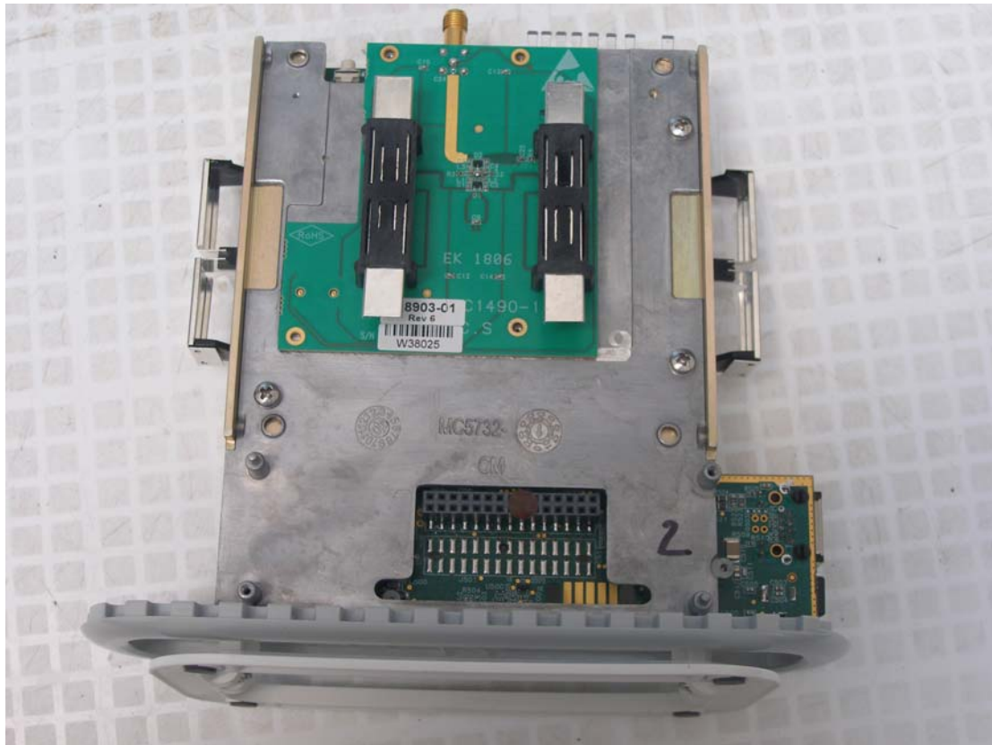
Photo9. CPE Si internal view, antennas
