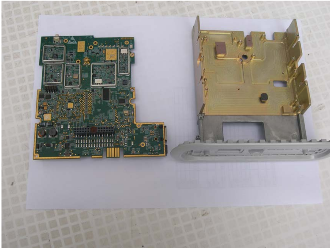
Photo4. CPE Si internal view PCB and frame
