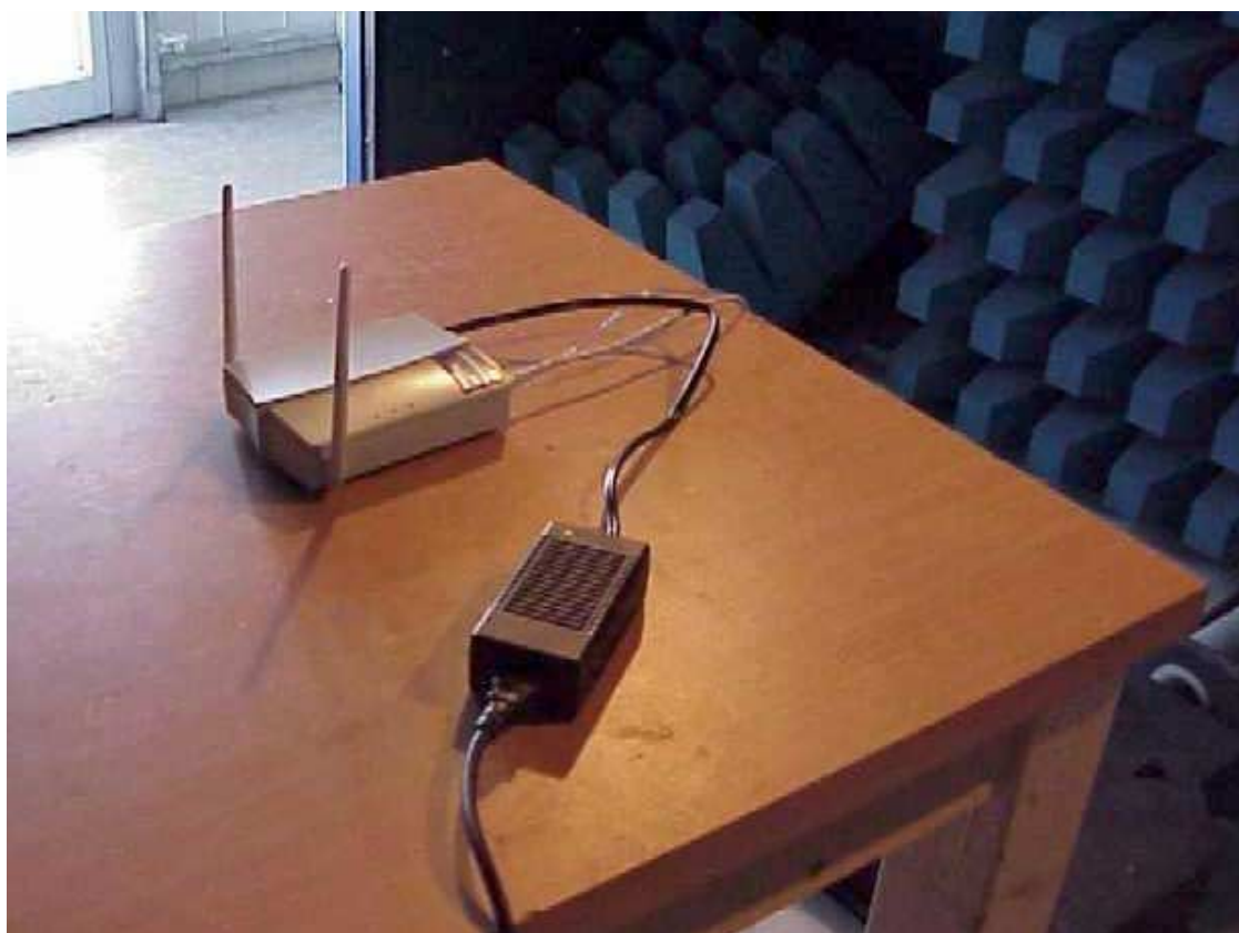
Photo #10 6dBi Omni antenna test configuration
