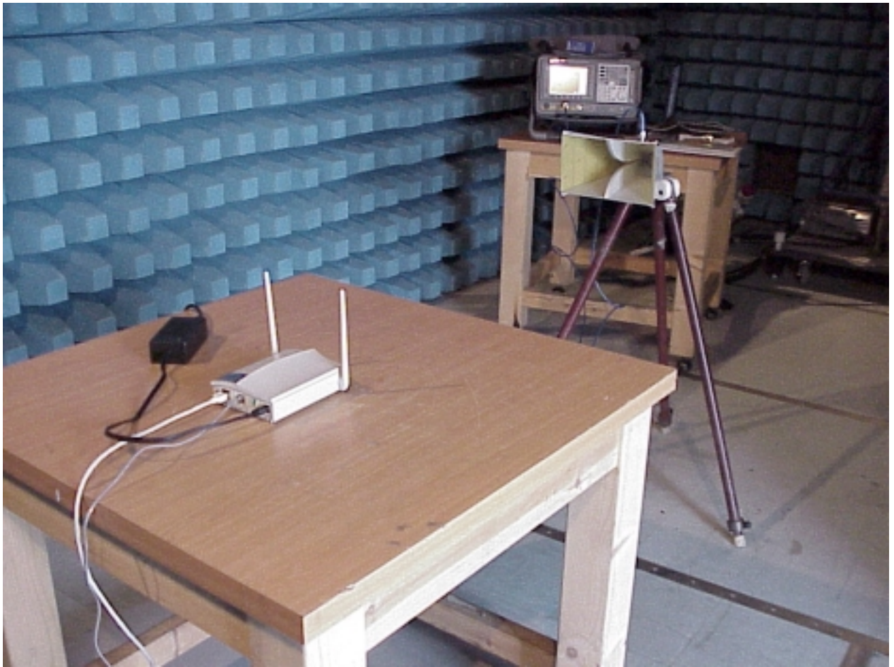
Photo #8 6dBi Omni antenna test configuration
