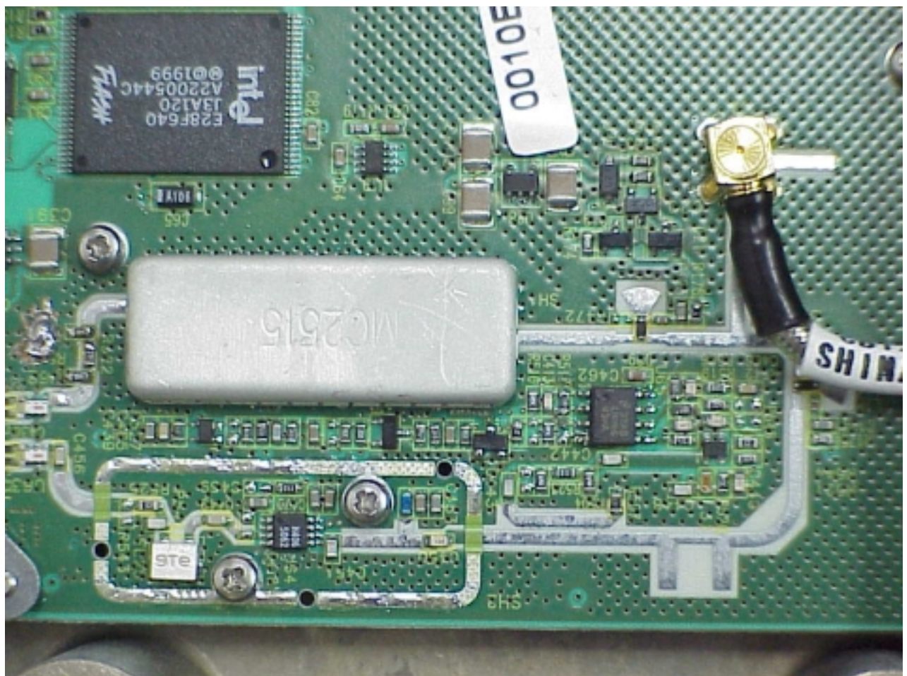
Photo 2 Radio Unit. Redesigned area (PWB component side)
