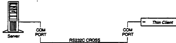
Direct Connection through RS232
