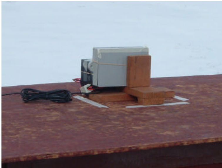
PICTORIAL 1 HEXAGRAM MODEL 10051M FIELD STRENGTH OF SPURIOUS EMISSIONS TYPICAL TEST SETUP
