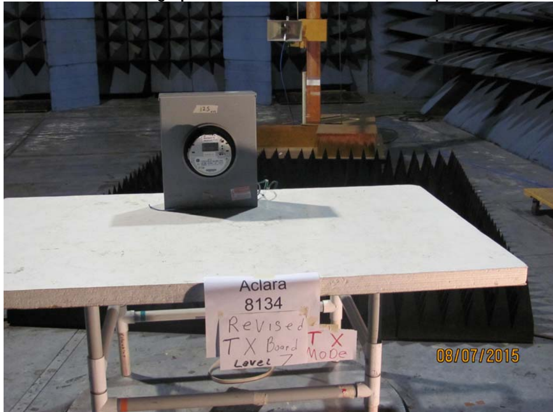
Photograph of Radiated Emissions Test Setup
