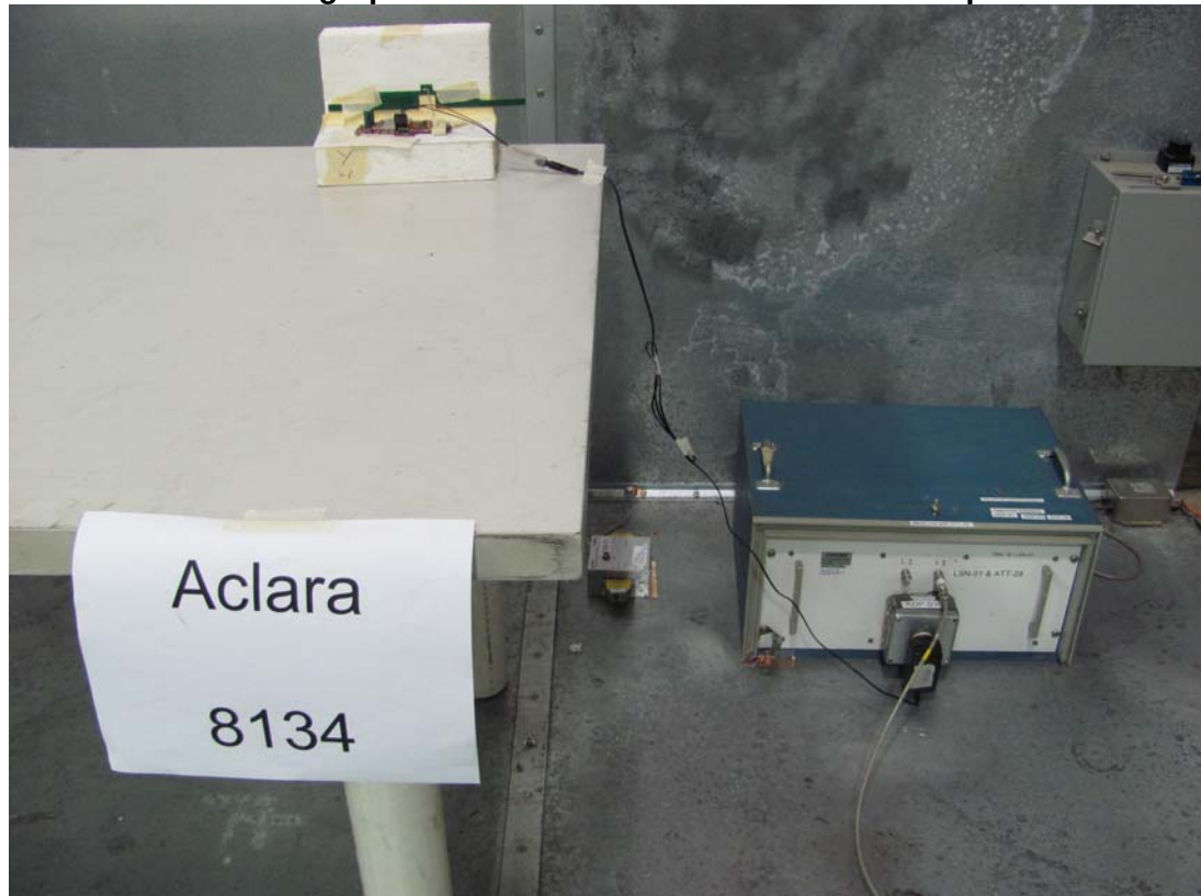
Photographs of Conducted Emissions Test Setup
