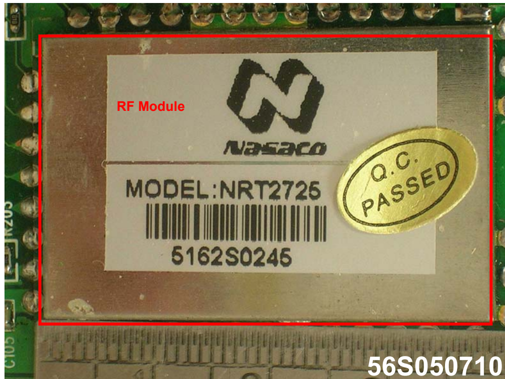
RF Module Circuit with RF Shield
