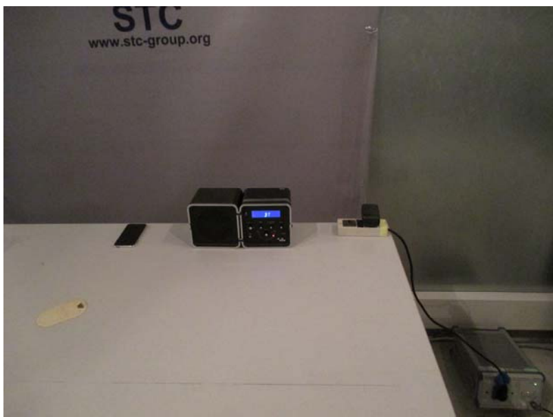
Measurement of Conducted Emission Test Set Up
