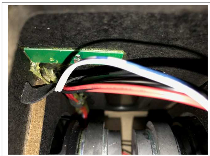
Internal Configuration 15 (Location of Wi-Fi Antenna)
