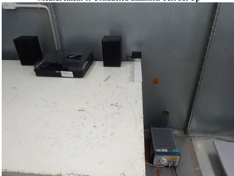
Measurement of Conducted Emission Test Set Up
