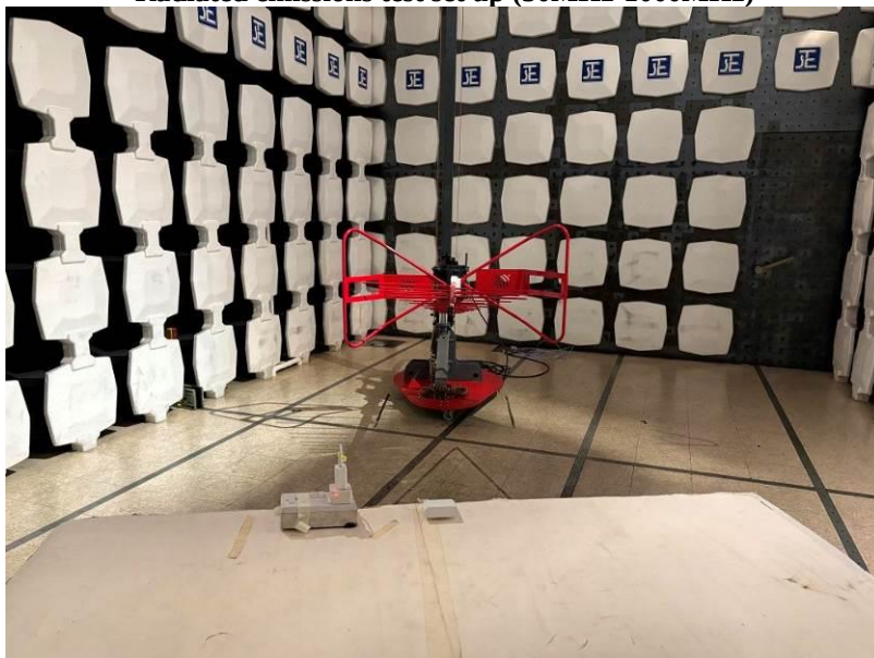
Radiated emissions test set up (30MHz-1000MHz)
