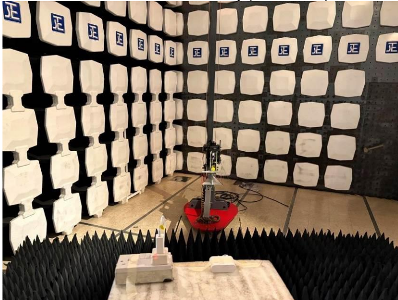
Measurement of Conducted Emission Test Set Up
