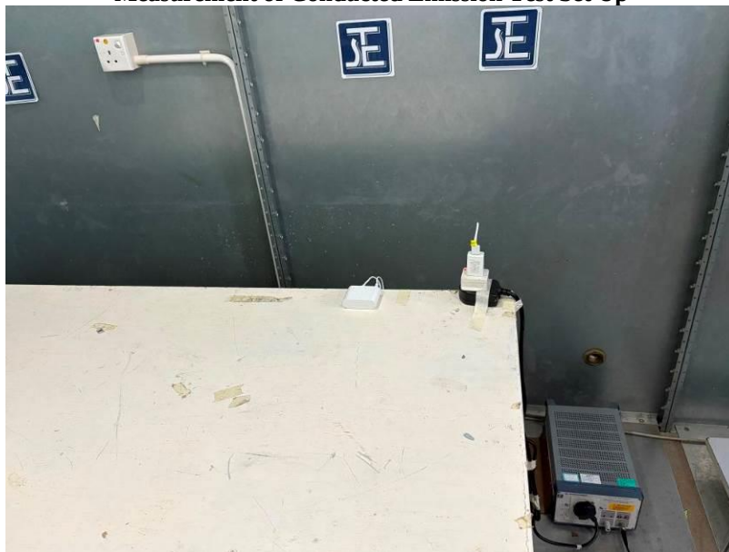
Measurement of Conducted Emission Test Set Up
