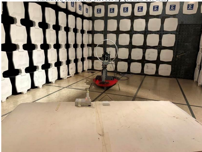
Radiated emissions test set up (9KHz-30MHz)
