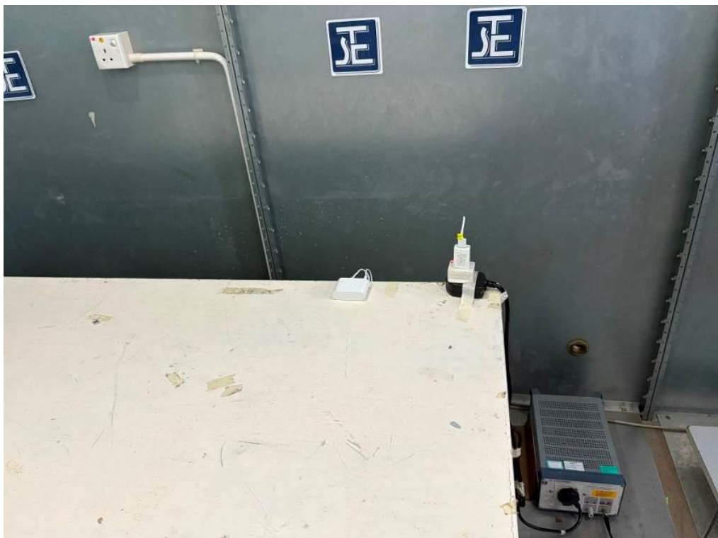
Measurement of Conducted Emission Test Set Up
