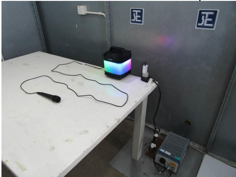
Measurement of Conducted Emission Test Set Up
