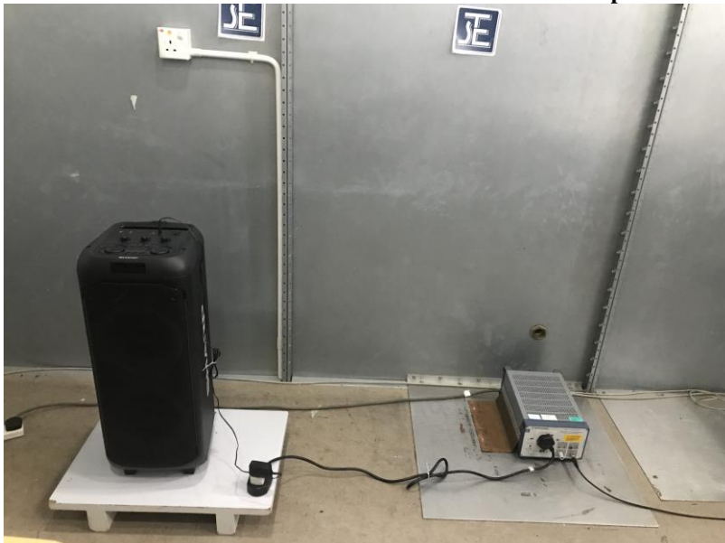
Measurement of Conducted Emission Test Set Up
