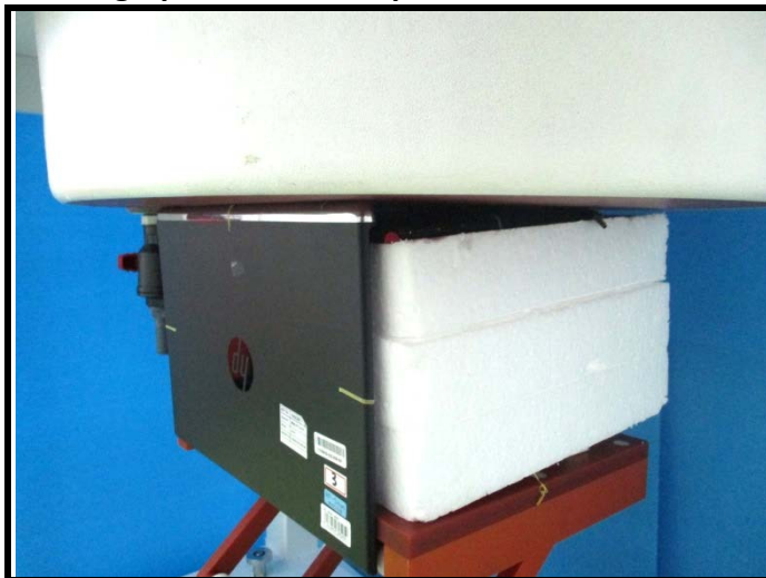
Bottom of EUT with 0 cm Gap
